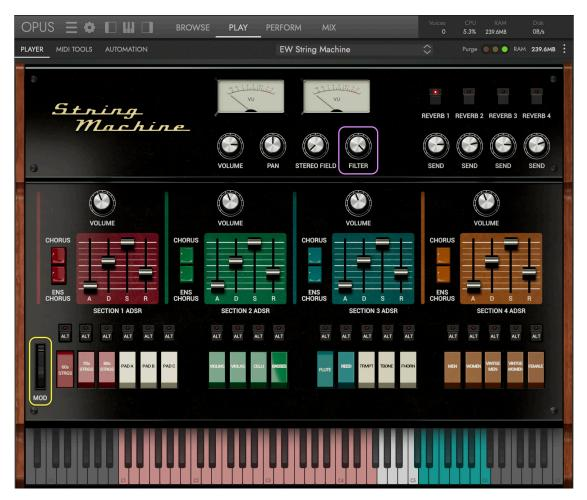
The **FILTER** CONTROL located in the Global Controls section is a macro parameter that simultaneously controls the filter cutoff on the Auto Filter effects inserted on each of the 4 instrument section's mixer channels. Program a MIDI controller to send Expression (CC 11) data to control this macro parameter in real-time.
