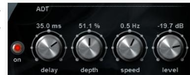
The **Delay** knob specifies in milliseconds, the delay between the original signal and the secondary signal. A delay of around 40 ms is typical, so is often a good starting point when crafting a specific effect.
